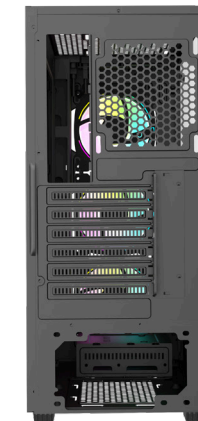
Front: 3 RGB Fans Included (120mm) Rear: 1 RGB Fan Included (120mm)
